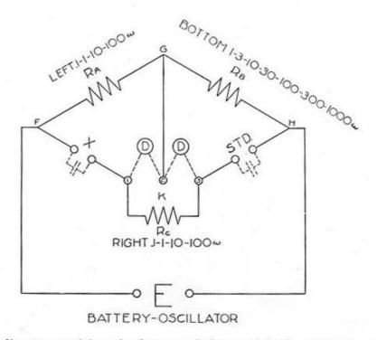
null indicator requiring simultaneous balance of both resistance and inductance. The solution of the network gives the equation for the unknown inductance
